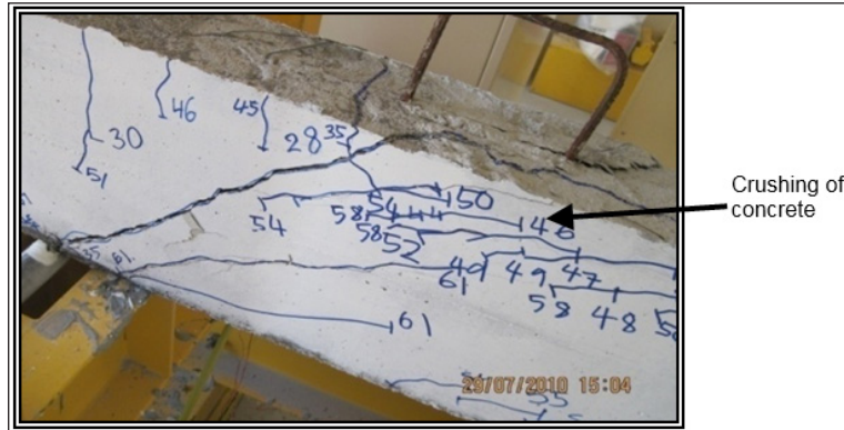
Figure 11. Crushing of concrete of Beam 3-0
