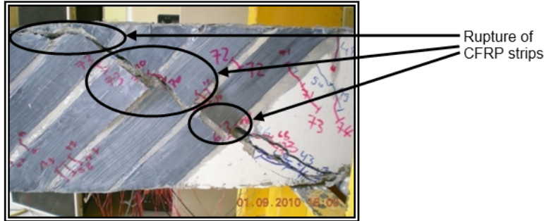
Figure 14. Shear failure of Beam 3-3 at a load of 325.39kN (shear force 110.63kN)
