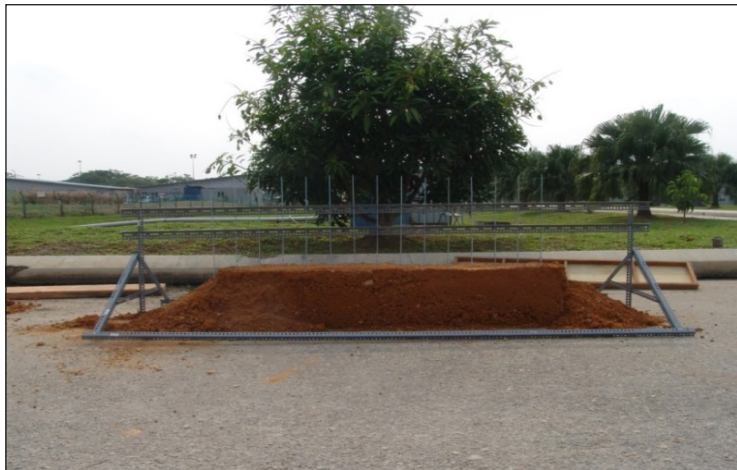
Figure 7. 15 rod steels in dexion structure was pointed respectively on the surface of the mini embankment to determine the initial reading before the moving load being imposed
