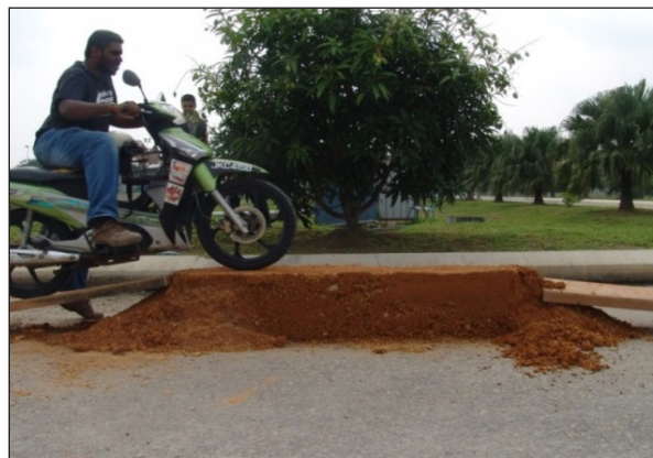
Figure 8. The platform was set at the two edges of mini embankment respectively and the motorcycle (moving load) was imposed through the mini embankment
