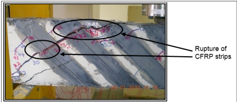
Figure 7. Shear failure of Beam 2-3 at a load of 411.25kN (shear force 134.68kN)
