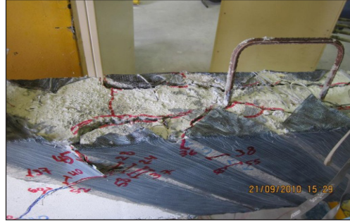
Figure 18. Splitting of concrete of Beam 3-4
